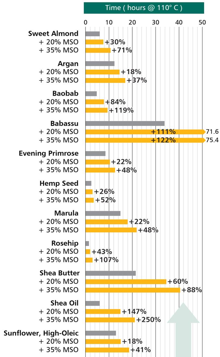
**Figure 2. Comparative OSI Values of Oils/Oil Blends**
